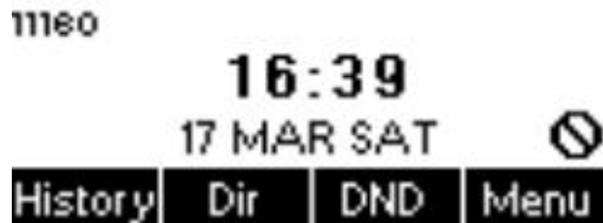
Figure 56 - DND Enabled on All Lines
